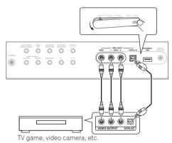
• Select these inputs by pressing **VIDEO** or using **INPUT SELECT** (remote) to select **VIDEO**.
